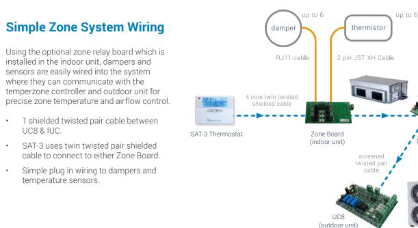
\* Important note: when designing a zoned system, the smallest zone must meet the minimum space requirements for R32 refrigerant.
